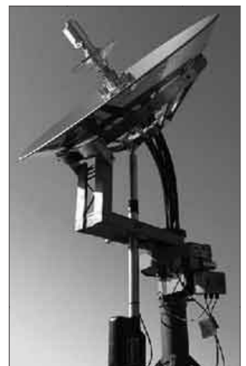
Figure 2. Solar collector mounted above pilot-scale bioreactor.
