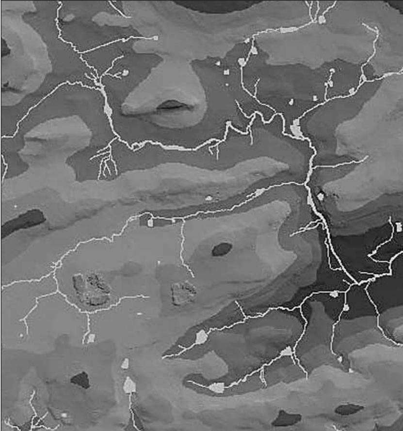
**GIS watershed model showing land elevation and stream drainage network.**
