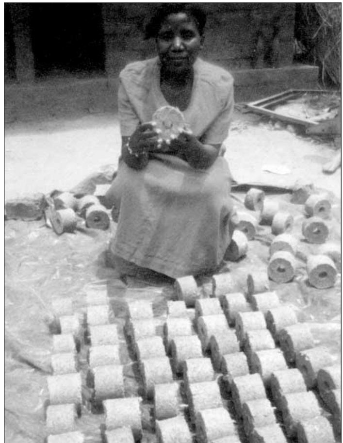
Use of briquettes can reduce the cutting of trees for fuelwood. The briquettes are made from agricultural waste which is compressed using a simple lever-operated press.
